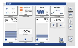
The display in the lower status bar changes from "ready" to "active". In the left bar graph, the ultrasonic dose appears and the docking indicator is active. The right bar graph shows the actual current flow. The treatment time is reduced by the second.
