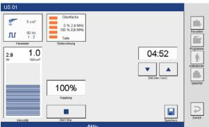
Touching starts the therapy. When therapy starts, the display in the bottom status bar changes from "Ready" to "Active "and the "Start" button changes to "Stop". In the bar graph, the configured dose is displayed and the therapy time counts down at one-second intervals. The coupling display is active.
