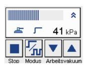
The intensity of the working vacuum is set via the two arrow keys. The bar graph shows the current value of the working vacuum.
