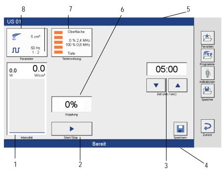
(1) Intensity The bar graph displays the currently set intensity. The intensity is adjusted using the left controller.
