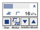
With activation of the basic vacuum, the vacuum is active. The bar graph shows the value of the basic vacuum.
