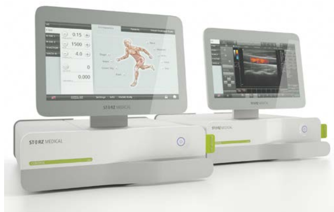
Control unit (15.6" touch screen) with optional diagnostic ultrasound
